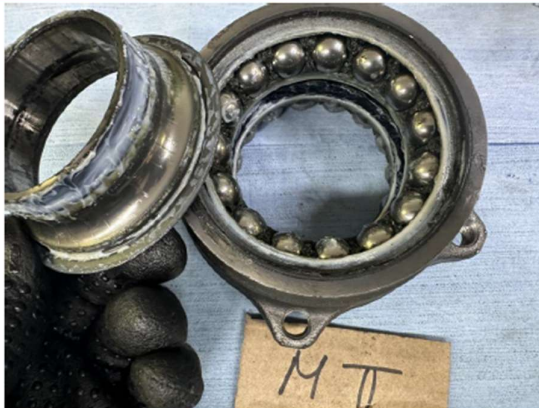
White grease in the M II bearing
