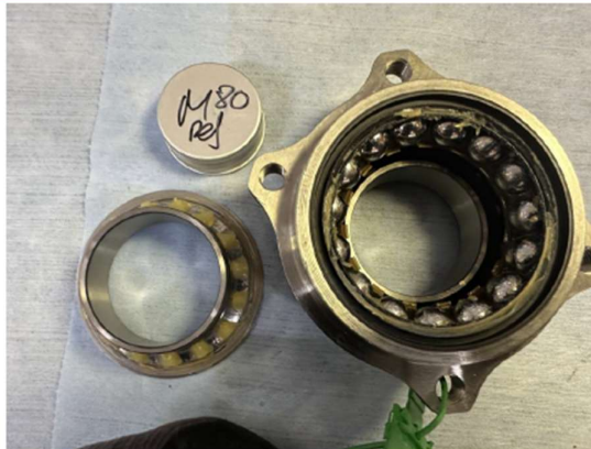
Honey colored grease in the M 80 reference bearing
